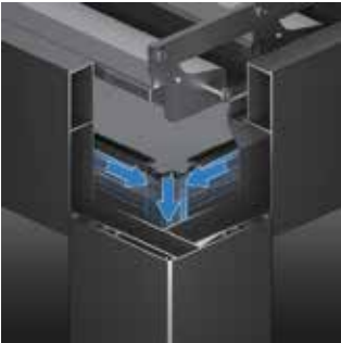
Water is routed through the post
